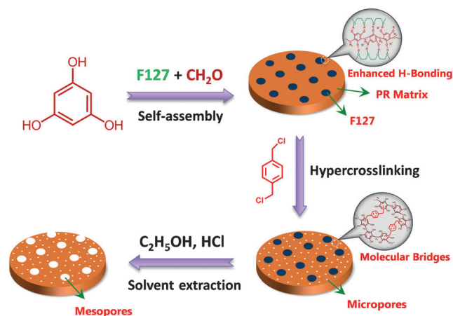
Scheme 1. Illustration of the synthetic process for Meso-PR basing on Friedel–Crafts alkylation reaction.
