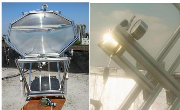
FIG. 1. Experimental system including the solar concentrator Fresnel lens (left) and the solar reactor (right).
